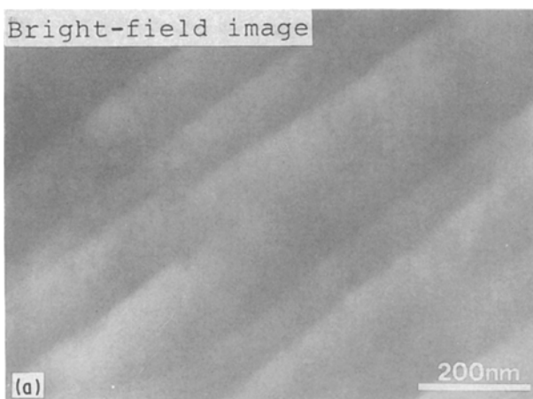
Figure 7 TEM images (a, b) and electron diffraction pattern (c) of an amorphous Al-15 at % Cr sample. The sample was ball-milled for 1000 h and heated to 740 K just after the first peak shown in Fig. 4
